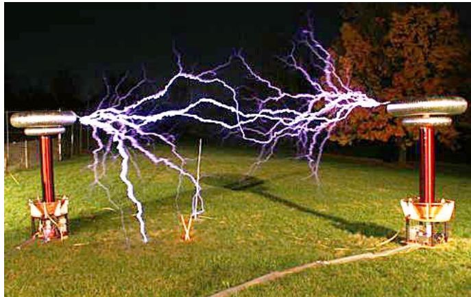
Breakdown voltage demonstration of two different materials conducting through an insulating medium, here, air 1
