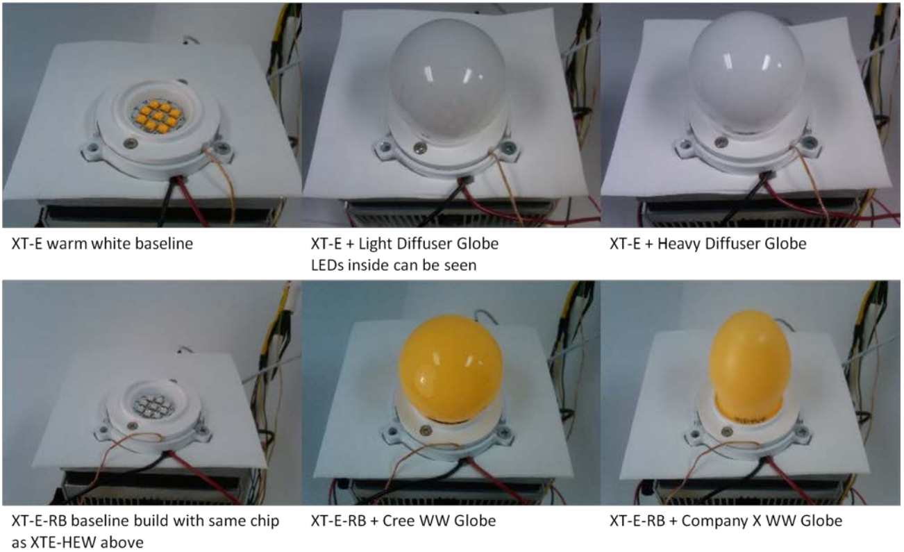
Fig. 4. Photographs of white LED and Remote Phosphor bulb test setups
